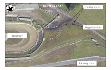
To achieve reliable measurements of both the raceway and speedway the logger location is elevated and is closer to the tracks than the legal boundary. However, testing has shown the noise logger records levels from the raceway that are approximately the same as the most exposed part of the site boundary. The raceway noise limits apply at this specific logger location and not at any other points on the site boundary.
